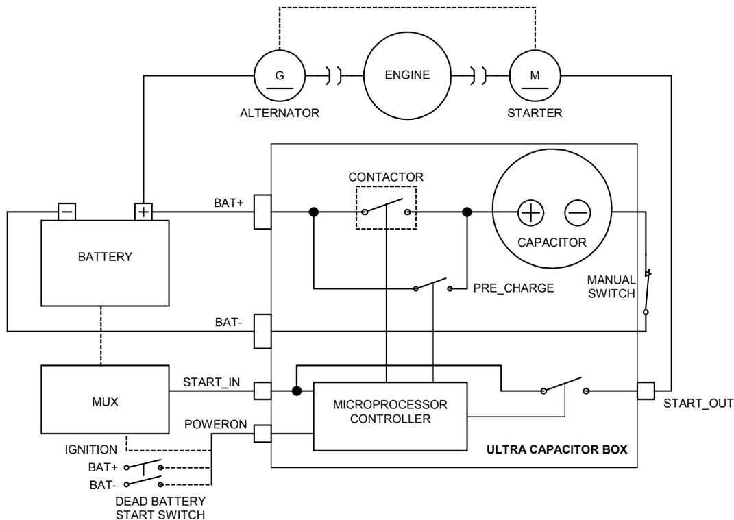
Figure 1. Block diagram of 80-kJ bus ultra capacitor system
